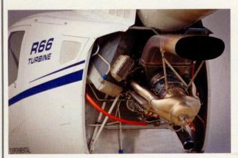
Located behind the exhaust stack, the engine has a cylinder shaped inlet barrier filter (not visible) with a bypass door should the filter become clogged. Inlet barrier filters have become popular with turbine-powered helicopters for their ability to protect the engine from fine dust and particles.
